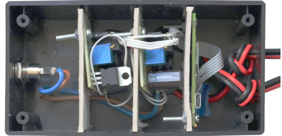
Fig. 5. The photo of the pattern generator and the LED drivers in the plastic enclosure.
