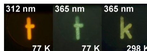
Fig. 14 Multicolour fluorescence image of our institutional logo ("ttk") visualized on temperature- and light-responsive microcrystals of 4 .
