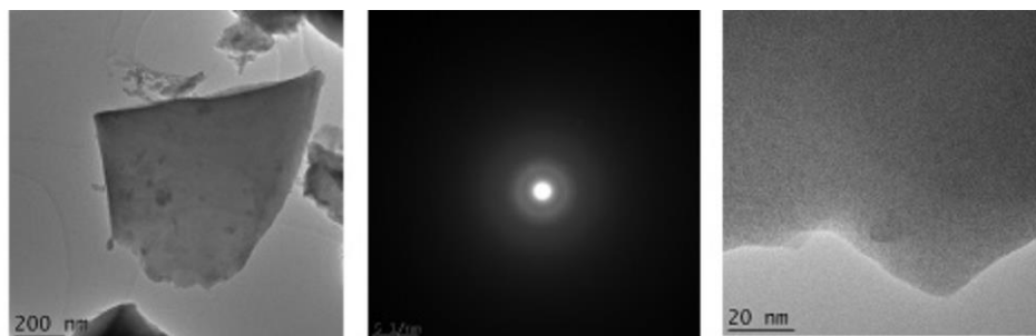
Figure 1. TEM images of 30\text{MoO}_3\text{-}50\text{ZnO}\text{-}20\text{B}_2\text{O}_3 glassy sample.
