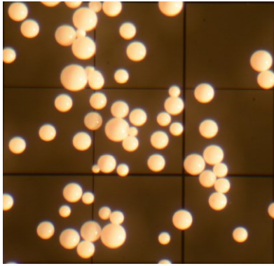
Small beads filled with cetyl alcohol covered by silica nanoparticles
