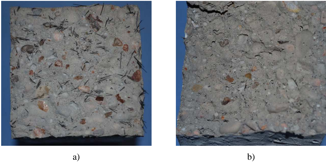
Figure 8: SFRC specimens after temperature loading (fiber content: 1.0 V%): a) cross-section of specimen failed in flexure, annealing temperature: 500 °C; b) cross-section of specimen failed in flexure, annealing temperature: 800 °C
