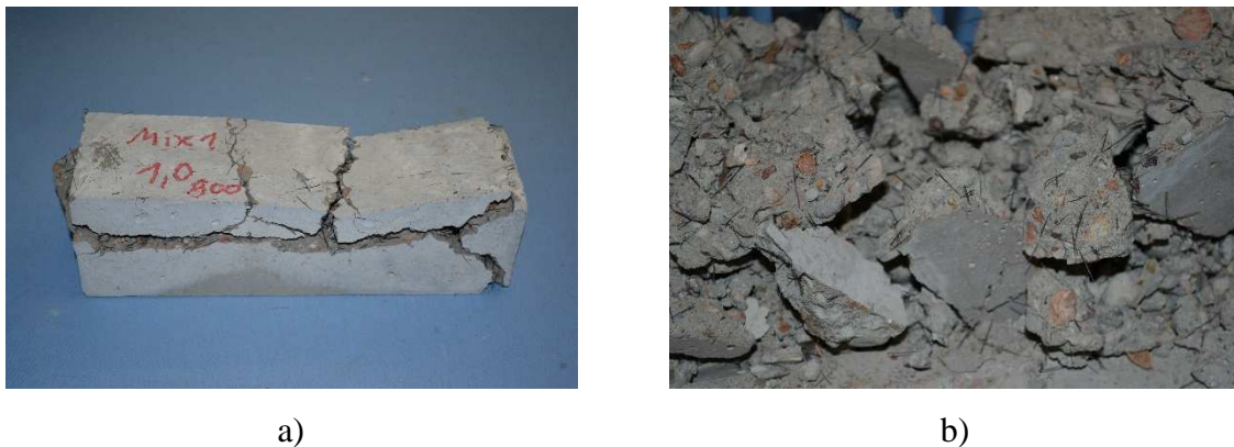
Figure 10: Explosive spalling of SFRC beam with 1.0 V% short steel fibers after annealing at 800 °C
