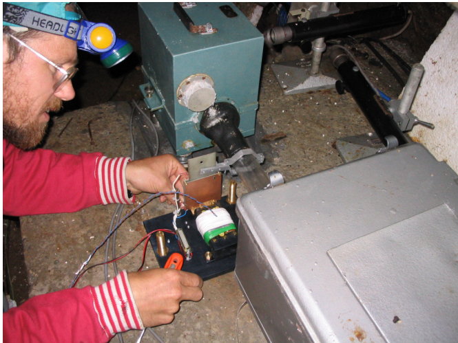
Fig. 7. In-situ calibration of the extensometer.
