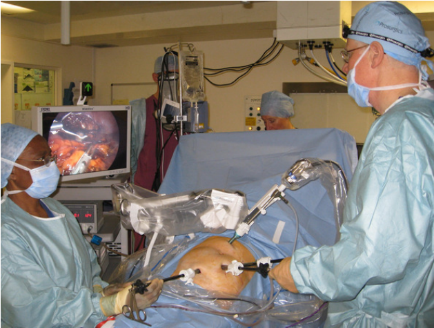
Fig. 2. Prosurge's FreeHand system during an operation. An infrared receiver is employed to pick up the head motions of the surgeon for camera control. (Image credit: Prosurge).
