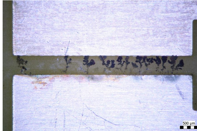
Fig. 5. Only dendrites formed in 0.1 mM \text{Na}_2\text{SO}_4 solution during WD test.
