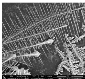
Fig. 1. Scanning electron microscope (SEM) image of dendrites.
