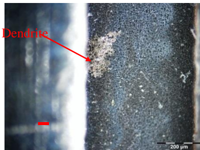
Fig.12. Dendrites were formed during the WD test using DI water.
