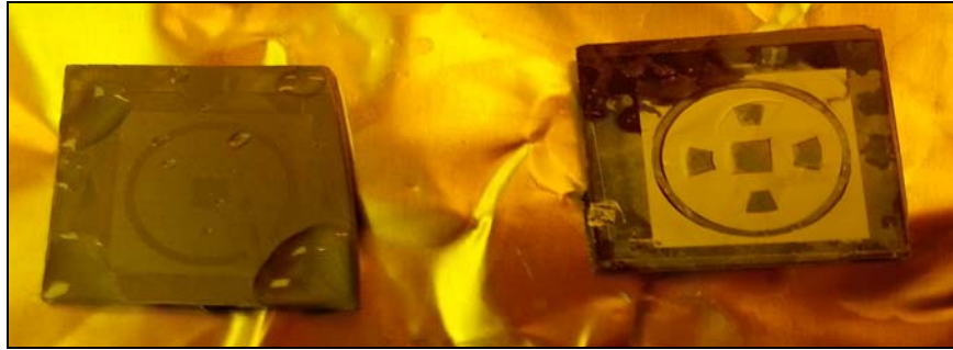
Fig. 7: ProTEX PS Primer and ProTEX ® PSB layer is deposited for MEMS capacitive pressure sensor diaphragm
