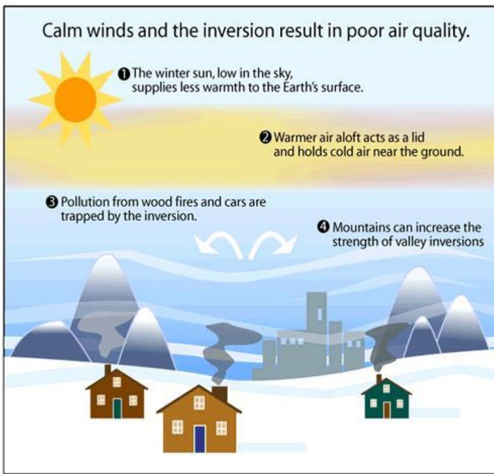
Figure 2.3: Temperature Inversion and the Effects. (US Environmental Protection Agency, 2011)
