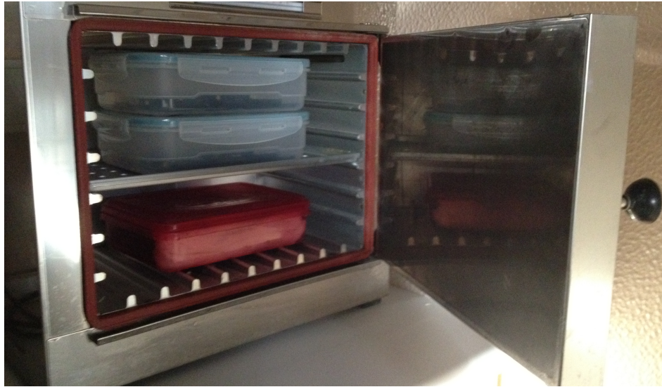
Figura 6 - Specimens were stored in distilled water for 48 h at 37°C.
