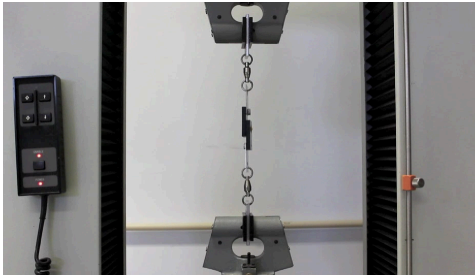
Figura 7 - SBS test in an universal testing machine Instron model 4502
