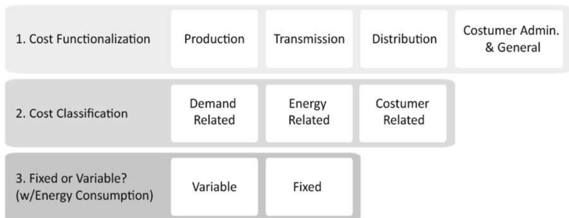
Figure 17 - Utility Cost Classification (Source: Adapted from NARUC 1992)
