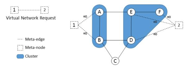
**Figure 2.5:** Augmented substrate graph with meta-nodes and meta-edges for a VNR. For each virtual node, it is created a meta-node that connects to a cluster of candidate substrate nodes, obeying location and capacity constraints. The connection between the meta-nodes and the substrate nodes is done through meta-edges with infinite bandwidth.
