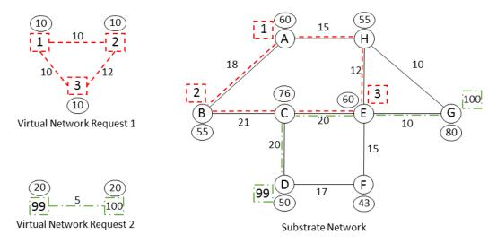
**Figure 2.4:** Embedding of multiple VNRs onto a shared SN. The circular shapes near the nodes in all networks are node parameters, i.e., CPU demand for virtual nodes and CPU available for substrate nodes. The numbers near the links are link parameters, i.e., bandwidth demand for virtual links and bandwidth available for substrate links. It is important to note that virtual links can be allocated to multiple substrate links (a path) in the SN.
