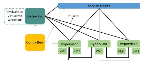
**Figure 2.1:** General architecture of NVP. Controllers manage the forwarding state of all hypervisors, gateways and service nodes. Gateways connect the logical networks with workloads on non-virtualized servers and service nodes are used for logical multicast or broadcast.
