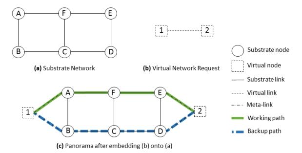
**Figure 3.2:** (a) Simple substrate network. (b) Simple virtual network request that arrives to be embedded. (c) Example of an embedding result of (b) onto (a) after the execution of our MILP formulation (supposing that all constraints are achieved - resource capacity, security, cloud type and dependability constraints).
