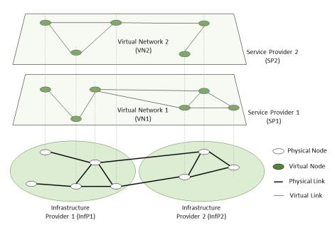
**Figure 1.1:** Network virtualization environment, with the SN at the bottom and one or more VNs on top. VNs are mapped onto the physical network. VNs can create a VN hierarchy, on which some architectural attributes can be inherited.
