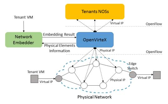
**Figure 2.2:** OVX system architecture. The IP translation is done at the edge switches for data packets and between OVX and the NOS for control packets.
