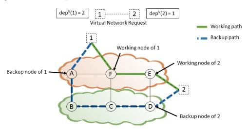
Figure 3.10: Example of an embedding respecting the  $dep^V$  required by the virtual nodes.
