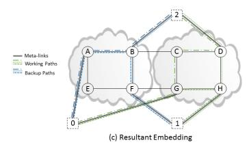
Figure 3.11: Example of a full embedding of a VN onto a SN with our solution.
