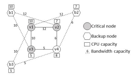
Figure 2.7: Representation of a K-redundant VN graph.
