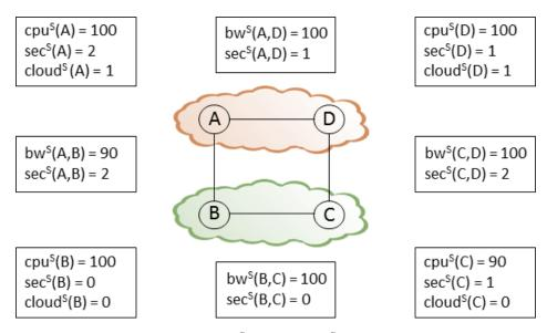
**Figure 3.3:** Example of a SN  $G^S$  where  $N^S = \{A, B, C, D\}$  and  $E^S = \{(A, B), (B, C), (C, D), (D, A)\}$ . The sets  $A_N^S$  and  $A_E^S$  (i.e., the attributes of the substrate resources) are presented in the figure.
