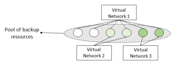
Figure 2.8: Pooling backup nodes. The backup nodes can be used by several VNs.
