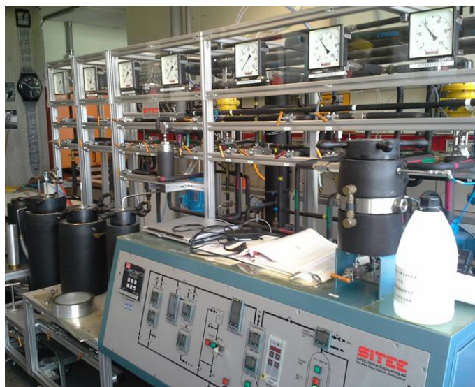
Figure 2.9 – Pilot unit designed for high-pressure extraction (RESS-technique).
