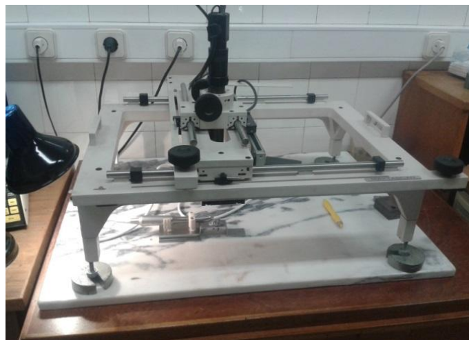
Figure 11 – X-Y coordinates measuring table where the mechanical system was set and where all instruments were measured after fracture.
