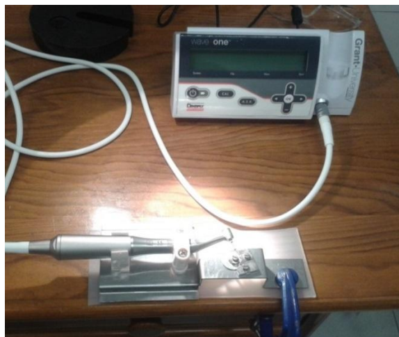
Figure 10 - Experimental assembly with the WaveOne™ motor
