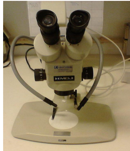
Figure 3.11 Stereomicroscope (Meiji Techno EMZ-8TR)
