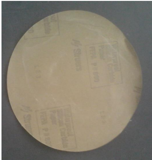
Figure 3.10. 800-grit polishing disk (Buehler II, Germany)
