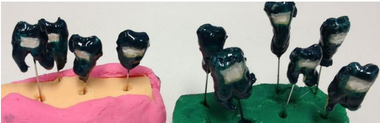
Figure 3.8 Specimen isolation with nail polish
