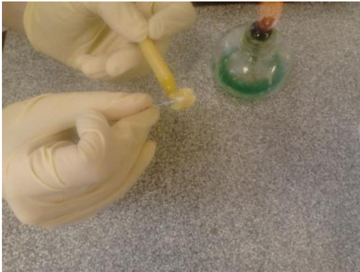
Figure 3.7 Specimen isolation with Sticky wax
