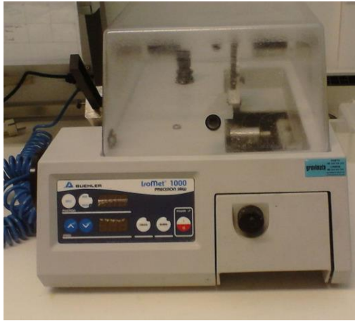
Figure 3.2. Precision Saw machine (IsoMet® 1000 Precision Saw from Buehler, Illinois, USA).
