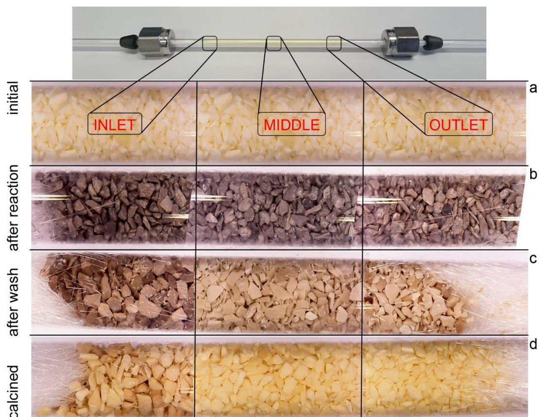
Figure 3.8 Photograph of the \text{CeO}_2 catalyst at three different locations along the axial direction of the catalyst bed: a. before the reaction, b. after the DMC synthesis for 35 h and a short (5-10 s) methanol washing at room temperature to remove the crystallites (Figure 3.6), c. subsequent methanol washing at 120 °C for 1 h, and d. after calcination of (c) under the flow of air at 300 °C for 12 h
