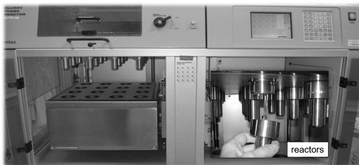
Figure 2.4 AMTECH SPR16 slurry phase reactor for high throughput experimentation
