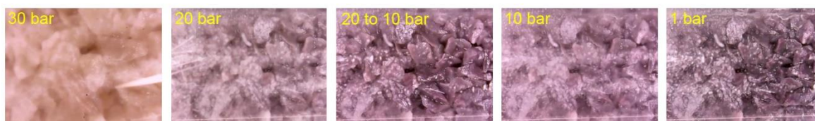
Figure 3.12 Operando visualization of the CeO 2 catalyst during the DMC synthesis from CO 2 and methanol in the presence of 2-CP. The experiment was started under the optimized reaction condition (30 bar, 120 °C) and the reaction pressure was lowered. The darker color at lower pressures is caused by the time-sequence of the experiment
