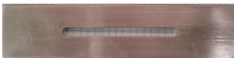
Figure 3.2 Home-made Al cover plate for the reactor furnace with ca. 6 cm channeling to allow the recording of the experiments
