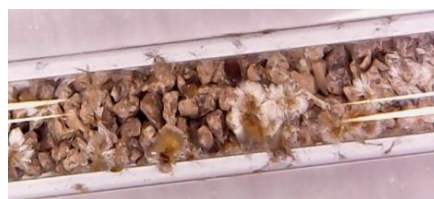
Figure 3.6 Photograph of the CeO 2 catalyst in the fused quartz reactor after 24 h of the reaction and subsequent drying
