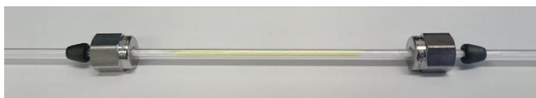
Figure 3.1 Fused quartz reactor with regular compression fittings. Fresh \text{CeO}_2 catalyst is loaded inside the reactor
