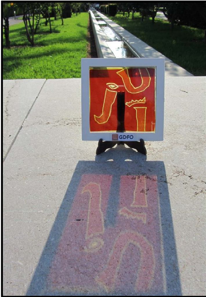
Figure 7.15: 10x10 cm 2 DSC with the logo of Universitat Jaume I with i_{sc} \approx 160 \text{ mA} and V_{oc} \approx 0.7 \text{ V} .
