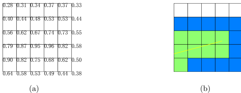
Figure 4.5: (a) A subarea of a Cartesian mesh with the phase field d values marked at the nodes. These values are the equivalent phase field values of the crack shown in yellow in (b) with \ell = 2\sqrt{2}a where a is the side length of the elements. (b) Schematic showing the effect of Algorithm 6: The set of elements E_0 (with d_{\text{crit}} = 0.6 ) is shown in either green or blue, and the set E is shown in green. The crack path will be sought in the green region. It can be seen that some elements, even though with a nodal point having a d value of 0.82, are not retained per (4.6).
