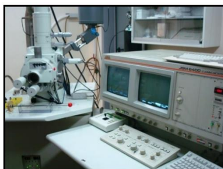
Figure 2.13 SEM equipment used for obtaining surface images
