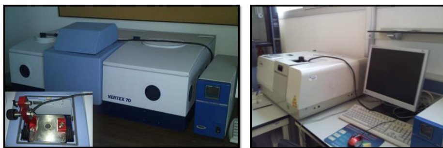
Figure 2.6 FT-IR devices used
