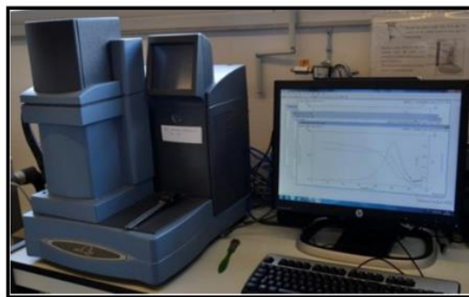
Figure 2.7 DMTA equipment used to study the viscoelastic properties
