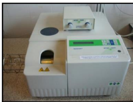
Figure 2.10 Thermobalance used for the thermal stability evaluation
