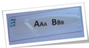
Figure 3. Photograph of one of the hybrid samples obtained showing the transparency of the coating
