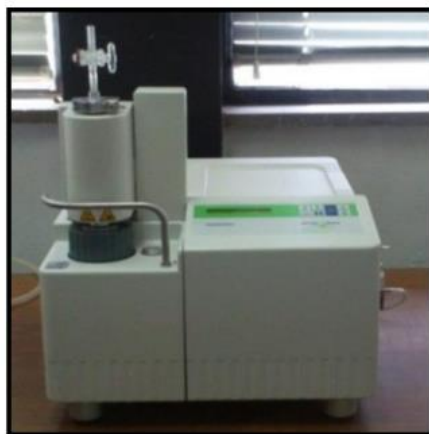
Figure 2.8 TMA apparatus used to perform thermomechanical analysis
