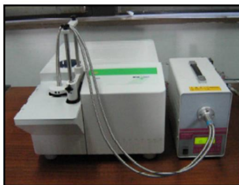
Figure 2.5 Photo-calorimeter used to perform photo-DSC experiments
