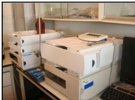
Figure 2.2 GPC chromatograph used for the molecular weight determination
