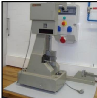
Figure 2.15 Impact testing machine used for the determination of the impact strength
