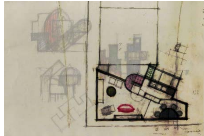
House in Yokohama: working sketches. The staircase as a articulating device between old and new is one of the prominent concerns shown in these drawings
