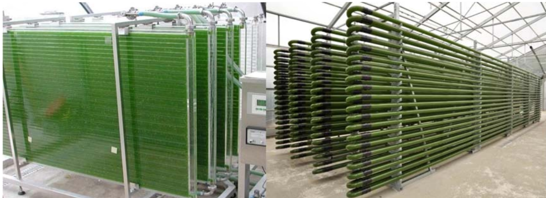
Image 1.2 Microalgal closed photoreactors. Top: vertical column; Bottom left: flat panel; Bottom right: horizontal tubular.
