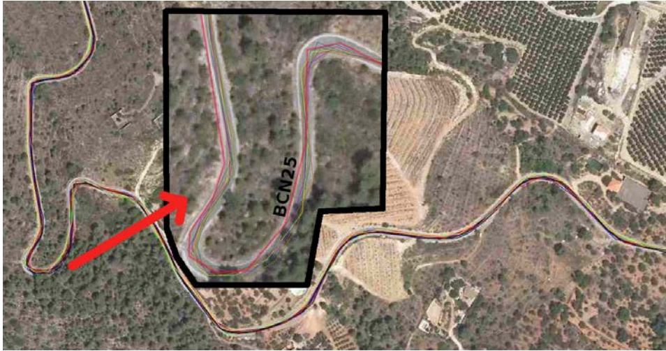
Figure 4.2: Micro-experiment. The wide red line is the official data. The thinnest lines are the digitalized ones.
