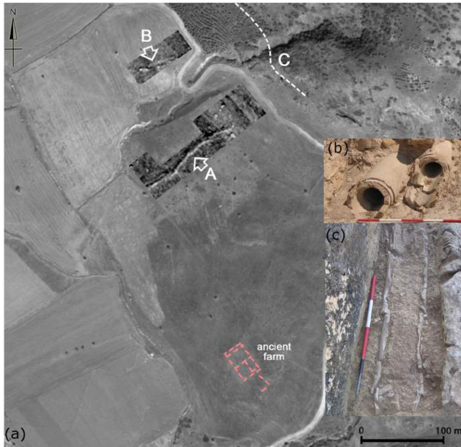
Fig. 15. (a) 2005 QuickBird panchromatic image of ROI A where geomagnetic maps have been overlaid. Magnetic anomalies (A–B) are, in terms of shape and dimensions, ascribable to buried terracotta pipes of an ancient aqueduct. To the Northeast of A and B, where geomagnetic investigations were performed, some pipelines are visible as seen in Fig. 15c. Pink dashed lines indicate the fabric of the farm, (b–c) Examples of terracotta pipe aqueducts in the territory of Hierapolis. In particular, the picture (c) shows a terracotta pipe found at the north-east of the surveyed areas. (For interpretation of the references to colour in this figure legend, the reader is referred to the web version of this article.)
