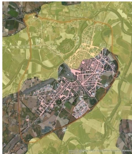
Figure 3.8: Alessandria - Area at risk (yellow: 500-year floodplain; orange: open spaces constituting the urban grid)
