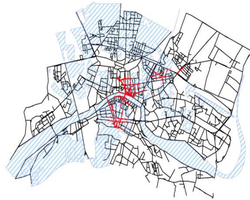
Figure 3.41: Pisa - Local integration core at risk (black: segment map; red: global integration core (R= 400M); blue: area at risk)
