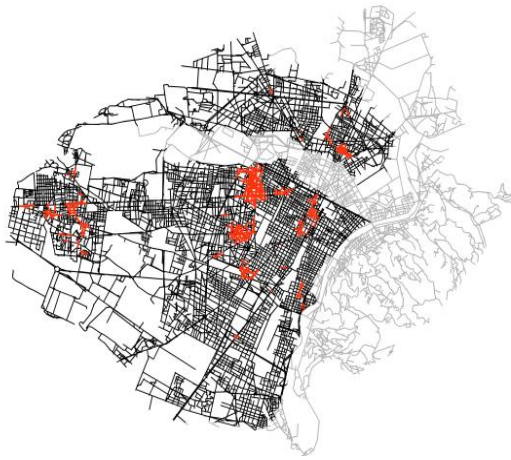
Figure 3.96: Torino- Scenario 1 , local integration core (R= 400m) (black: segment map; red: local integration core (R= 400m); grey: segments within flooded area)
