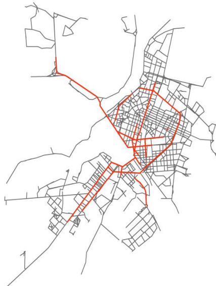
Figure 3.7: Alessandria - Global Choice core (R = n) (black: segment map, red: 10% highest values)
