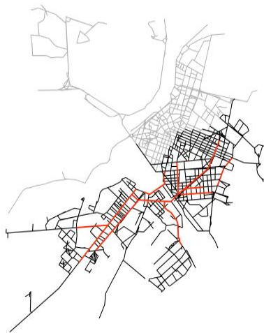
Figure 3.25: Alessandria - Scenario 1, global choice core (R= n) (black: segment map, red: global choice (R= n); grey: segments within flooded areas)
