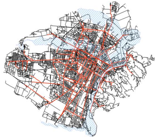
Figure 3.99: Torino- Scenario 0 (black: segment map; red: global choice core (R= n); blue: area at risk)
