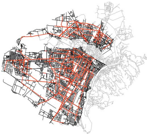
Figure 3.98: Torino- Scenario 1 , global choice core (R= n) (black: segment map; red: global choice core (R= n); grey: segments within flooded area)
