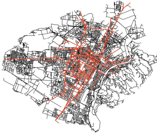
Figure 3.77: Torino -Global integration core (R = n) (black: segment map; red: 10% highest values)
