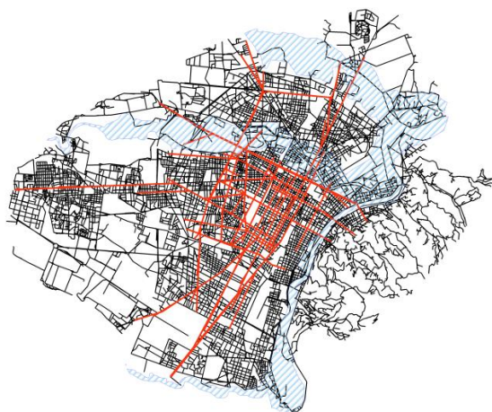
Figure 3.81: Torino - Global integration core at risk (black: segment map; red: global integration core (R= n); blue: area at risk)
