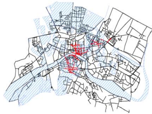
Figure 3.56: Pisa, Scenario 0 (black: segment map; red: local integration core (R= 400m); blue: area at risk)
