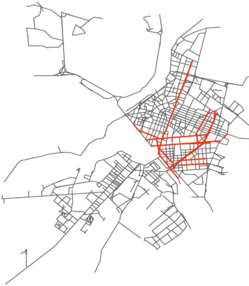
Figure 3.5: Alessandria - Global integration core (R = n) (black: segment map, red: 10% highest values)
