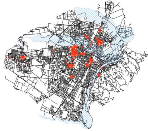
Figure 3.97: Torino- Scenario 0 (black: segment map; red: local integration core (R= 400m); blue: area at risk)
