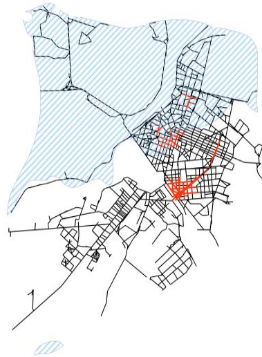
Figure 3.10: Alessandria - Local integration core at risk (black: segment map, red: local integration core (R= 400m), blue: area at risk)
