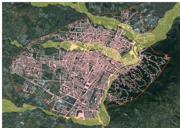
Figure 3.80: Torino - Area at risk (yellow: 500-year floodplain; orange: open spaces constituting the urban grid)
