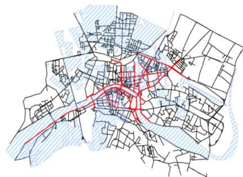
Figure 3.54: Pisa - Scenario 0 (black: segment map; red: global integration core ( R= n ); blue: area at risk)
