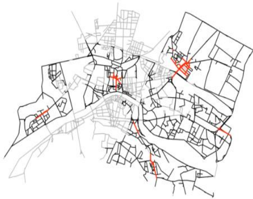
Figure 3.55: Pisa - Scenario 1 , local integration core (R= 400m) (black: segment map; red: local integration core (R= n); blue: area at risk; grey: segments within flooded area)
