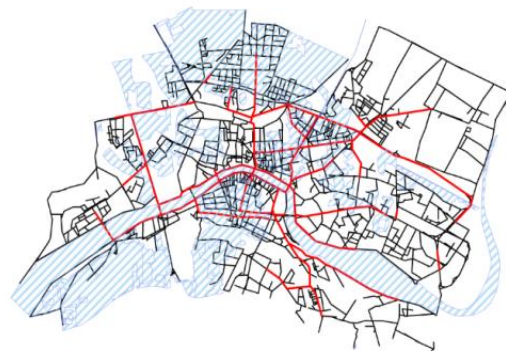
Figure 3.58: Pisa, Scenario 0 (black: segment map; red: global choice core (R= n); blue: area at risk)
