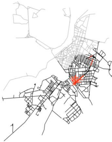
Figure 3.23: Alessandria - Scenario 1, local integration core (R= 400m) (black: segment map; red: local integration (R= 400m); grey: segments within flooded areas)
