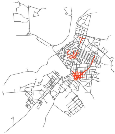
Figure 3.6: Alessandria - Local integration core (R = 400m) (black: segment map, red: 10% highest values)
