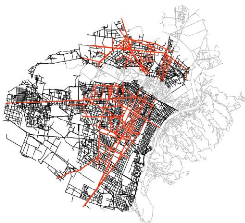
Figure 3.94: Torino - Scenario 1 , global integration core (R= n) (black: segment map; red: global integration core (R= n); grey: segments within flooded area)
