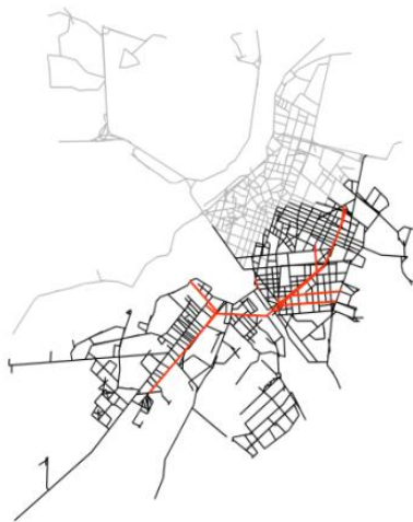
Figure 3.21: Alessandria - Scenario 1, global integration core (R= n) (black: segment map; red: global integration core (R= n); grey: segments within flooded areas)
