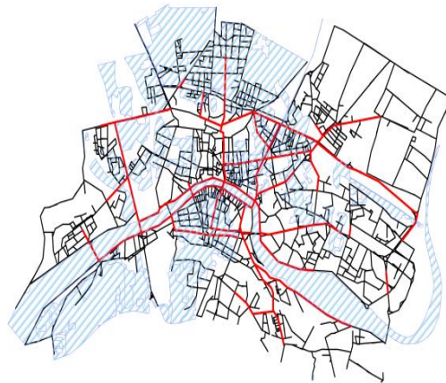
Figure 3.42: Pisa. Global choice core at risk (black: segment map; red: global integration core (R= n); blue: area at risk)
