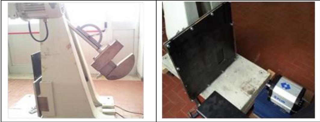
Figure 1: Impact tests setup. (left) Charpy pendulum , (right) specimen lodge and position of the infrared camera
