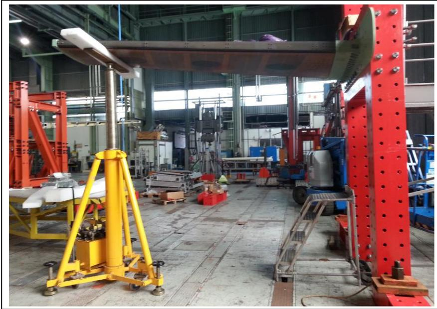
Figure 4.30: wingbox demonstrator in floating condition
