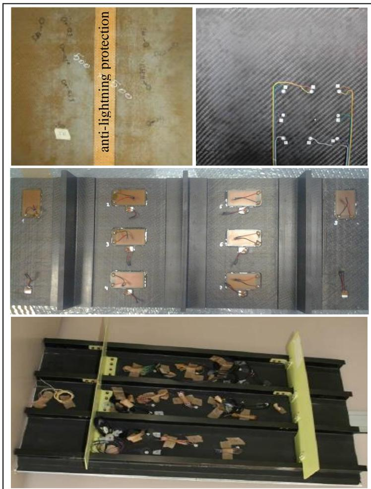
Figure 3.20: preliminary flat and stiffened panel analyzed
