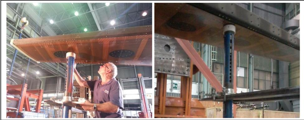
Figure 4.16: LWP impact energy test calibration
