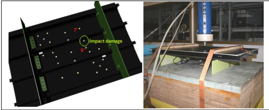
Figure 3.52: stiffened panel source and receiver PZT patches and impact locations (left), Alenia Aermacchi experimental impact test (right)
