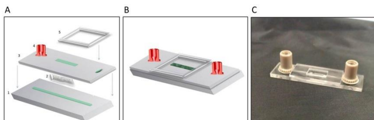
Fig. 8 Assembly of the PMMA microfluidic device.
