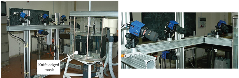
Figure 3.3 Pictures of the setup: tomographic experimental apparatus during the calibration procedure (left); camera arrangement: four 5.5 megapixels cameras LAVision Imager sCMOS.
