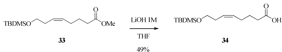
Scheme 3.24: Basic hydrolysis of ester 33 .
