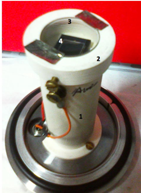
Figure 4.14: Picture of the quartz window mounted on the support. 1. Plastic Pillar, 2. Special mounting for the windows, 3. Quartz window, 4. NIST calibrated photodiode.
