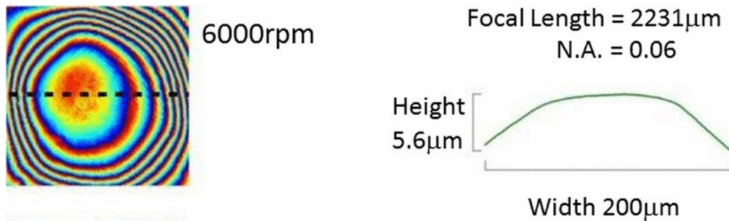
Figure 4.6: Phase maps (left) of single microlens made at 6000 RPM. The dashed lines correspond to reconstructed microlens profile shown on the right.
