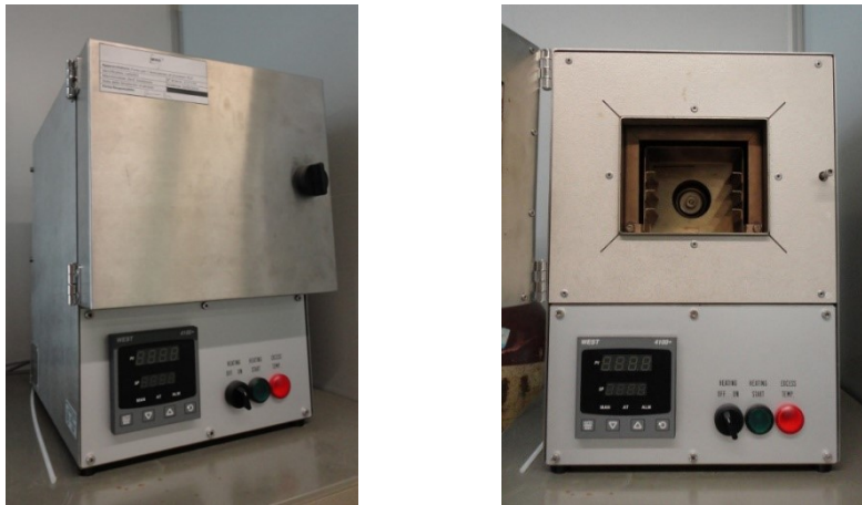
Figure 3.8. Oven used to the TLD annealing.
