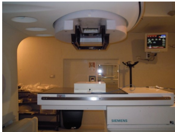
Figure 4.6. Picture of the set up for the measurement of the Primus Siemens accelerator output. PTW Farmer 3006 chamber was placed in a water equivalent slab phantom at 5 cm depth with a 1 cm backscatter slab. The photon beam was delivered setting 100 MU, 10 x 10 cm 2 square field, 100 cm of source to isocenter distance.
