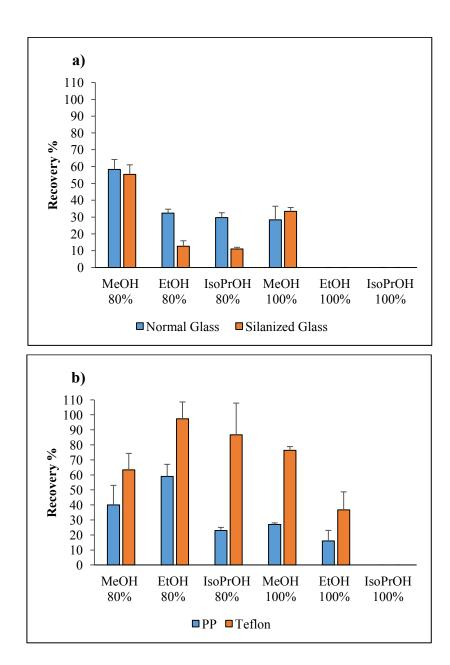
**Figure VIII.4** Recoveries of PLTX following complete drying in various solvents using both normal and silanized glass vials (4a) or PP and Teflon tubes (4b). Error bars represent standard deviation (n= 3)
