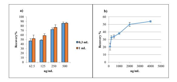
**Figure VIII.5** Recoveries of PLTX following complete drying in 80% aqueous MeOH at different spiking concentrations (62.5, 125, 250 and 500 ng/mL) and subsequent redissolution either in 0.3 or 1 mL of 50% aqueous MeOH (5a). Recoveries of PLTX following freeze-drying in 10% of aqueous MeOH at different spiking concentrations (125, 250, 500, 1000, 2000 and 4000 ng/mL) and subsequent re-dissolution in 0.3 mL of 50% aqueous MeOH (5b). Error bars represent standard deviation (n= 3)
