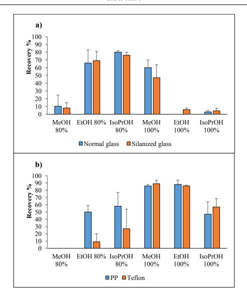
**Figure VIII.3** Recoveries of PLTX following concentration in various solvents using both normal and silanized glass vials (3a) or PP and Teflon tubes (3b). Error bars represent standard deviation (n= 3)
