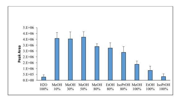
**Figure VIII.1** Chromatographic peak areas obtained from LC-HRMS analysis of PLTX 1:10 dilution in various solvents mixtures. Error bars represent standard deviation (n= 3)
