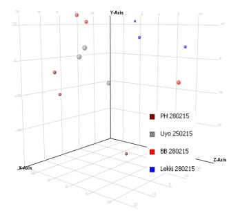
**Figure VI.8** Score plot of the principal component analysis of passive samples from all four sites (BB=Bar Beach, PH=Port Harcourt), all taken during week 9 of 2015 (n=3). The three principal components plotted on the X, Y, and Z axes account for ca. 66% of the total variability in the data set (39.04% for X; 18.79% for Y and 9.04% for Z)
