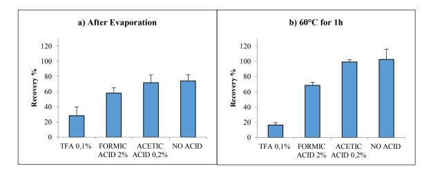
**Figure VIII.6** Recoveries of PLTX (125ng) following complete drying in three different 80% aqueous MeOH mixtures containing respectively 0.2% of acetic acid, 0.1% of trifluoroacetic acid and 2% of formic acid and subsequent re-dissolution in 1 mL of 80% aqueous MeOH (6a). Recoveries of the same PLTX acidic mixtures following a heat-treatment (60° C for 1 hour) (6b). Error bars represent standard deviation (n= 3)
