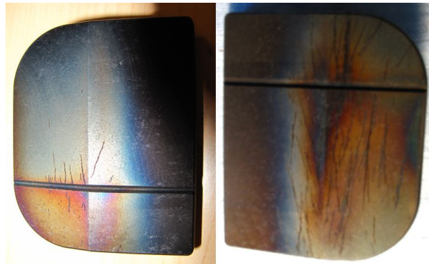
Figure 4.3.3: Outer (left) and inner (right) samples after exposure
