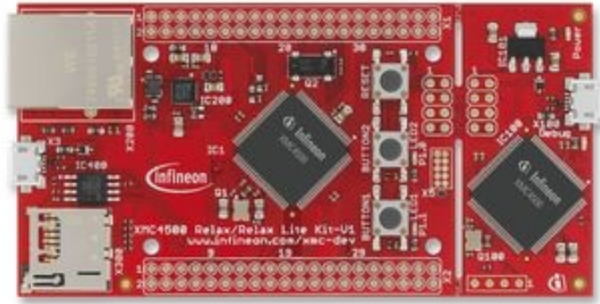
Figura 26: XMC4500 Microcontroller (ARM® Cortex™-M4F based)
