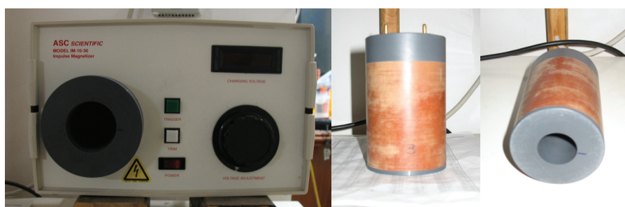
Figure 2.22: ASC Scientific IM-10-30 with coils
