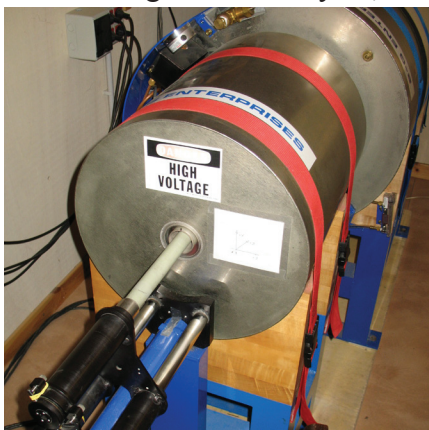
Figure 2.20: 2G Enterprises AF demagnetizer
