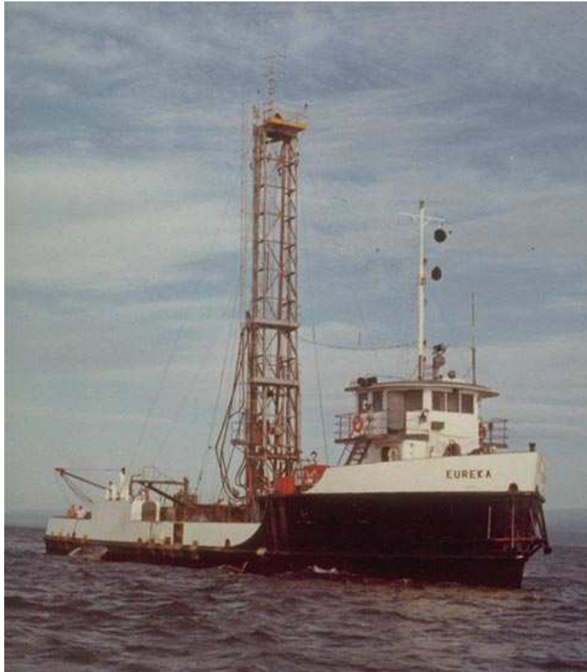
Figure 6 - Ship "Eureka", the first dynamic positioned vessel [20].
