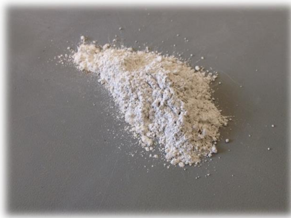
Figure 2.3: Physical appearance of Ground Granulated Blast Furnace Slag (GGBS) used in this research.
