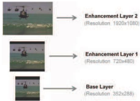
Figure 2.3: An example of spatial Scalability approach in H.264/SVC. Source: (Unanue et al., 2011b)
