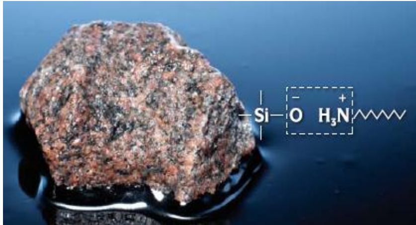
Plate 2.2: Interaction of Rediset with a Siliceous Aggregate (AkzoNobel, 2013)
