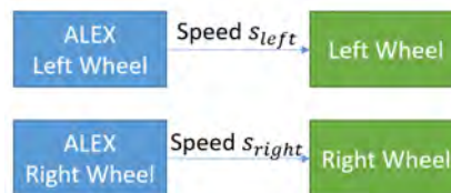
Figure 6.24 — The core of the rover architecture. Each ALEX controller is responsible of the speed of one wheel.
