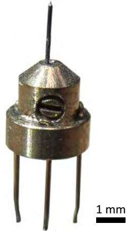
FIGURE 3.5 – Support for the sample (the "hat"), with a W wire inserted. At the top of the wire, a CCnT is attached (not visible).
