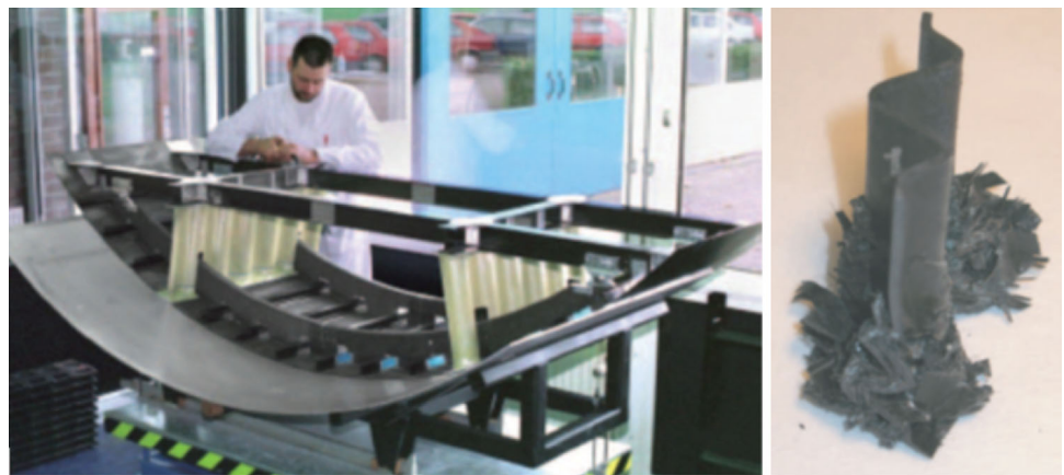
Fig. 1 Left Composite fuselage analysis [1]. Right Load buckling of some fronds [6]
