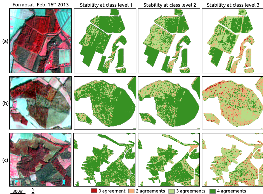
Figure 7. Degree of relative agreement between the SVM, RF, k-NN and GMM classifiers at the three classification levels using W_{bands} dataset. Stability is observed at level 3 for monospecific tree plantations in (a) compared to complex forests with mixed pixels in (b) and (c).
