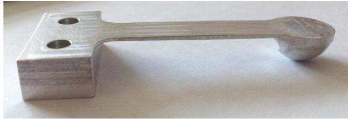
Figure 3.14 The passive layer of prototype unimorph transducer “II”. The actual passive layer is integrated with the base and the indentation half-sphere for the sake of simpler structure
