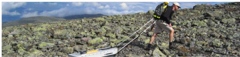
(b) GPR used in location without vehicle access ( http://www.malags.com/solutions ).
