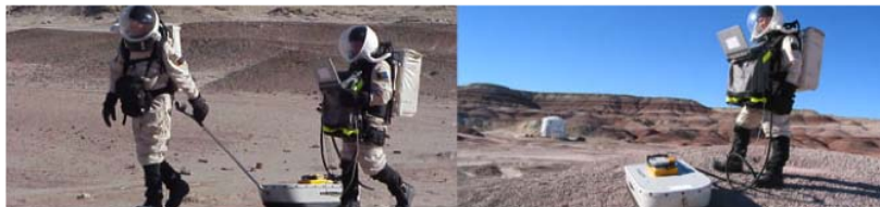
(c) GPR used in hazardous environments ( http://www.malags.com/solutions ).
