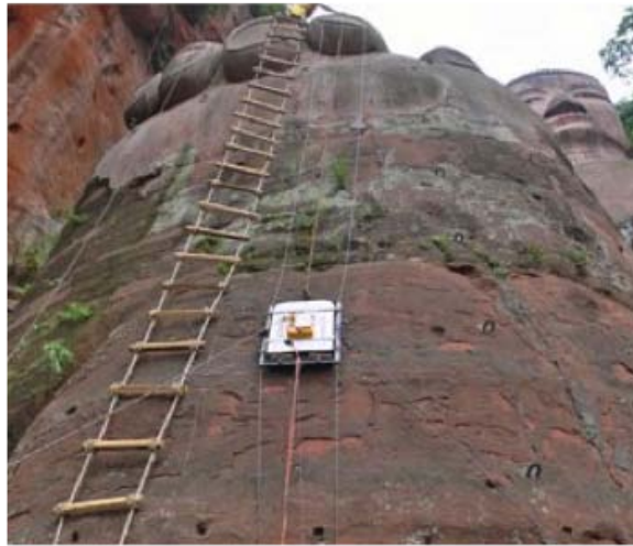
(a) GPR sytem in verticql configuration ( http://www.malags.com/solutions ).
