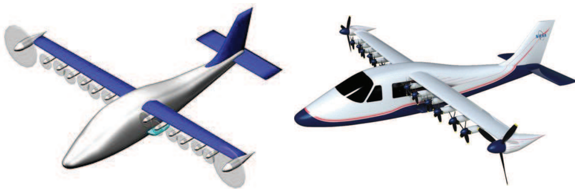
Figure 9. SCEPTOR 8,9 . NASA's Distributed Electric Flight Demonstrator Project.
