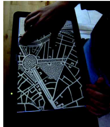
Figure 2. Touch the map! allows blind users to interact with a tactile map and retrieve names, distances and details using gestural interaction technique. Retrieved from (A. Brock et al., 2010).
