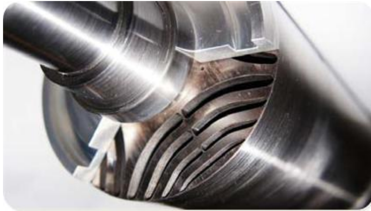
Fig. 1.9 Synchronous reluctance machine rotor with 4-pole configuration [23].
